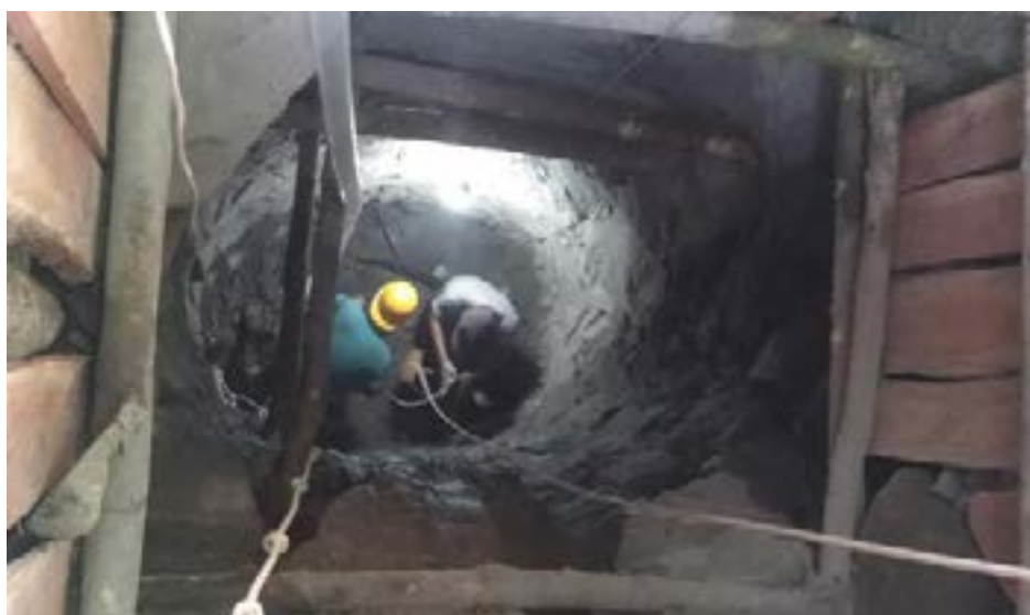
Fig. 12: A vertical shaft in a 200 × 200 foot mining plot (Fig. 8) penetrated bedded carbonaceous rocks at Kyauk Tan Maw (Khamti mining area). This is a mine operated with our geological consultancy where the mine owner guaranteed total control over ethical issues.
