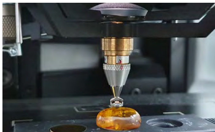
Fig. 4 A germanium ATR crystal was used with direct contact to the surface of the amber specimens. The method requires liquid nitrogen cooling for the microscope unit detector.
