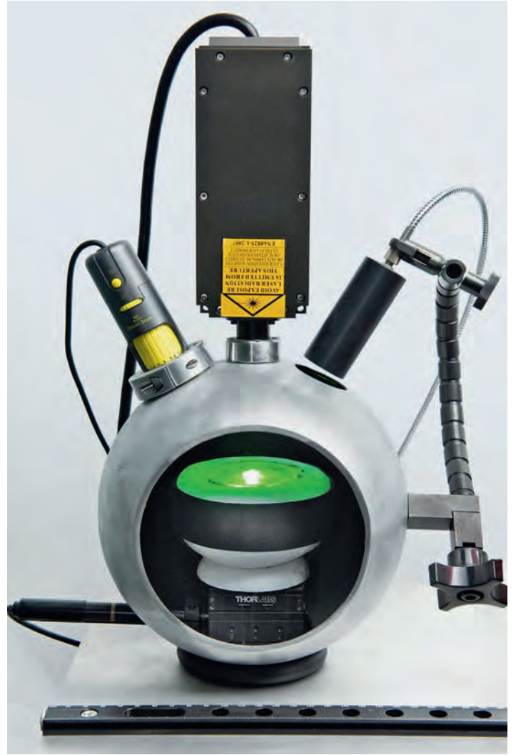
Fig. 5 A look at the GRS research laboratory instrumentation in Switzerland, Hong Kong and Thailand. On the left side the custom-built photoluminescence analysis system with 2 laser sources (405 and 532 nm) is shown. The right side shows a close-up of one analyzed head with a 532 nm laser illuminating a sample.
