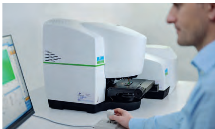
Fig. 3 Attenuated Total Reflection (ATR) spectroscopy for non-destructive analysis of amber in mm sample resolution at the Laboratory of GRS Thailand in Bangkok.
