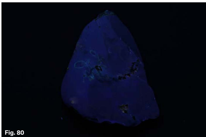
Fig. 78-81: Long-wave UV (365 nm), Fig. a) and b) and short-wave UV (254nm), Fig. c) and d) images of amber sample GRS-Ref-27746. The images were taken with a Canon EOS R camera using a 24-105 mm lens.
