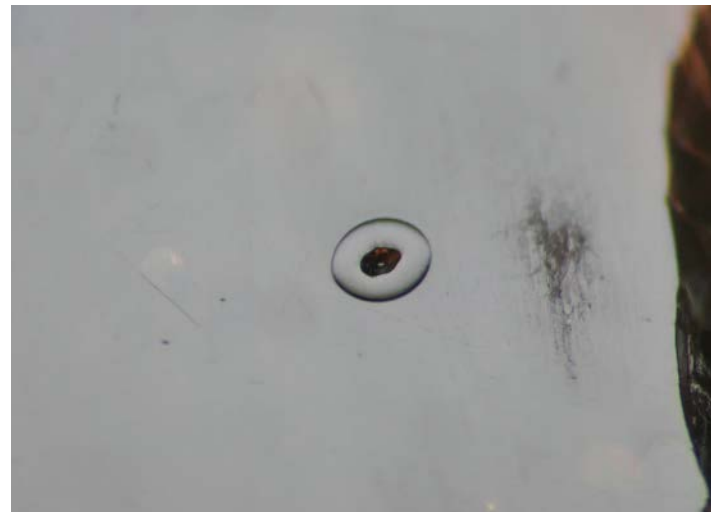
Fig. 6 Laser marks as a result of PL measurement with a 405 nm laser. After 5 seconds excitation GRS-Ref-28627-Oculudentavis naga. Diameter of crater is approximately 20 \mu\text{m} .
